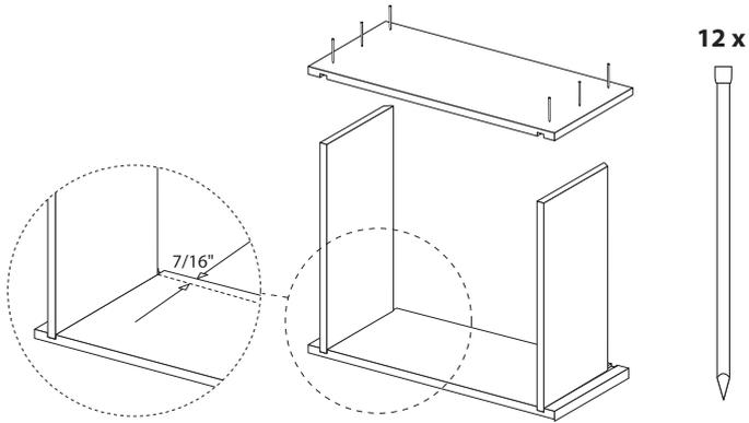
**1** Lay side panel flat. Insert support panels chamfer sloping down and outwards into rebates. The top edge must be 7/16" below the top edge of the side panel. Nail side panels to support boards using 12 x 40 mm lost head nails
