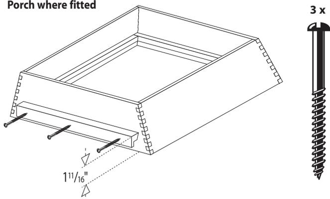
**3** Position porch base, correct way up as shown, with top edge  $1\frac{1}{16}$  inches above lower edge of lift. Fix in place with 3 x 40 mm black japanned screws.
