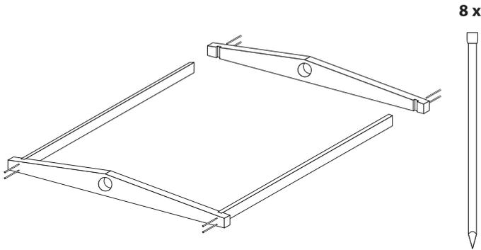
**1** Assemble roof ends to side rails sides as shown. Nail through ends into side rails using 8 x 40 mm lost head nails. Check assembly remains square.
