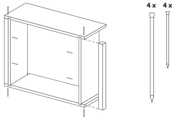
**2** Place side blocks in position, flush to corners as shown and nail in position using 4 x 25mm pins and 4 x 40 mm lost head nails
