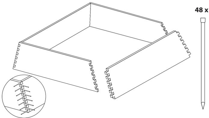
**1** Fit sides together as shown. Nail through each dovetail with a 40 mm lost head nail as shown in diagram, 12 per corner. Check assembly is square.
