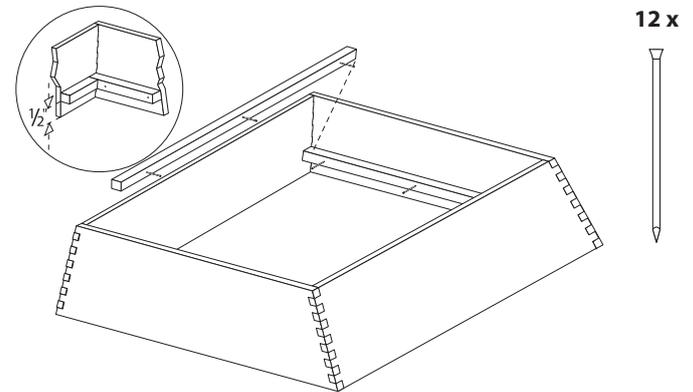
**2** Position lift support battens 1/2" up from lower edge as shown and nail each one with 3 x 25 mm pins.
