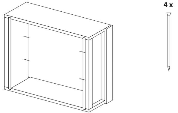
**4** Nail through side panels into side blocks using 4 x 25 mm pins, ensuring side blocks remain flush with lower edge of side strip.
