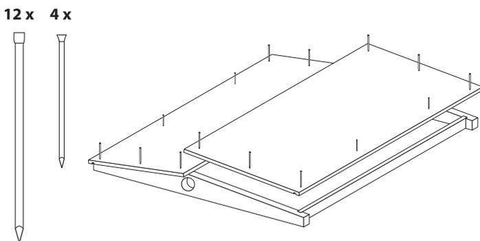
**3** Position roof panels as shown (overhang equally at each end) and nail to end boards using 12 x 40 mm lost head nails. Nail to sides using 4 x 25 mm pins.
