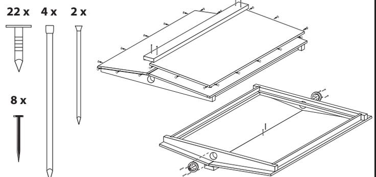
**4** Turn roof over, place metal covers over roof and nail to roof edges using 22 x 12 mm round head nails. Position apex cover strip as shown and nail to roof end boards using 4 x 40 mm lost head nails. Turn roof over and nail through roof panels into apex cover strip using 2 x 25 mm pins. Position vent covers over vent holes and nail in place using 8 x 12 mm black japanned round head tacks.
