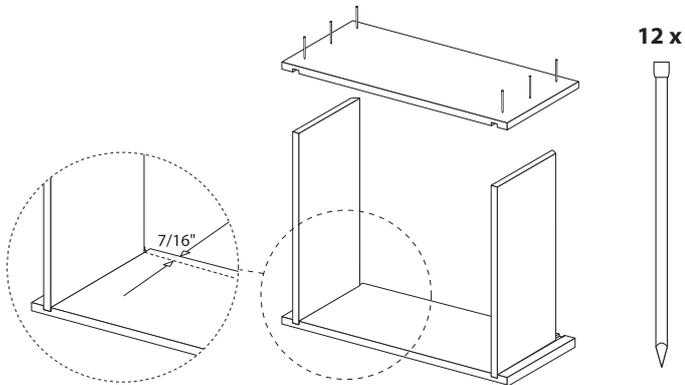
**1** Lay side panel flat. Insert support panels chamfer sloping down and outwards into rebates. The top edge must be 7/16" below the top edge of the side panel. Nail side panels to support boards using 12 x 40 mm lost head nails
