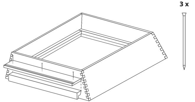
**4** Place porch roof with drip groove uppermost and outwards onto porch base and nail with 3 x 25 mm pins.
