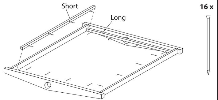
**2** Turn roof over and position inner end strips (longer). Nail to ends using 4 x 25 mm pins. Position inner side strips (shorter). Nail to sides using 4 x 25 mm pins.
