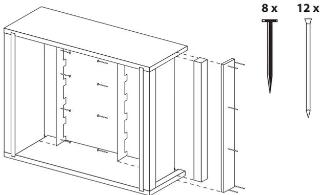
**3** Fit second pair of blocks between side panels and nail side strips to side panels, flush to top edge of side panels, using 12 x 25 mm pins. Fit Frame Separators to inside of side panels as shown, using 8 x 19mm frame nails.
