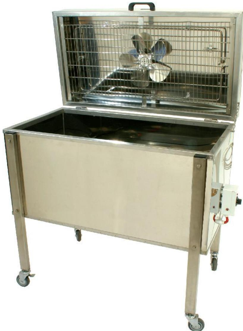
Before the machine is taken into use it is important to ensure that the machine is placed on a stable surface and the wheels are locked in order to keep it from rolling. The machine should be placed in a room with good lightning. This ensures safe and proper handling of the machine. The cord of the machine (230V) is to be placed so it minimises the chance for people stumbling over the cord during operation, cleaning and maintenance work etc. The machine is never to be left unattended during use.
